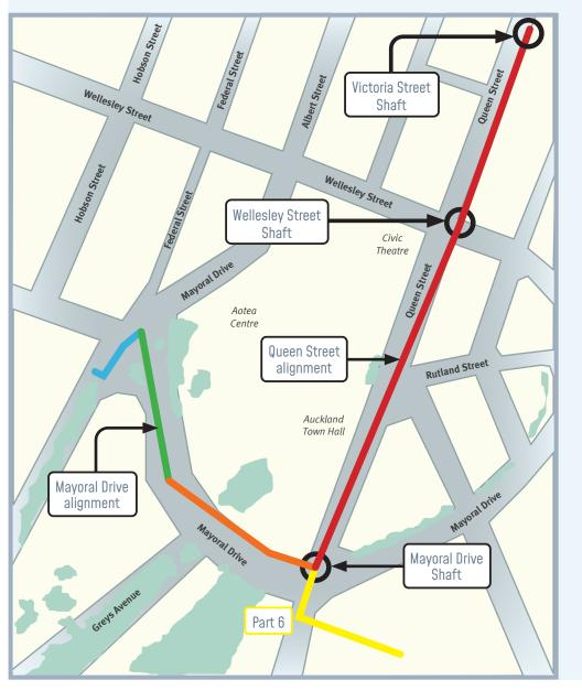
The Mayoral Drive Alignment will be constructed using a mix of open cut and trenchless construction while the Queen Street Alignment will be constructed using trenchless construction.
